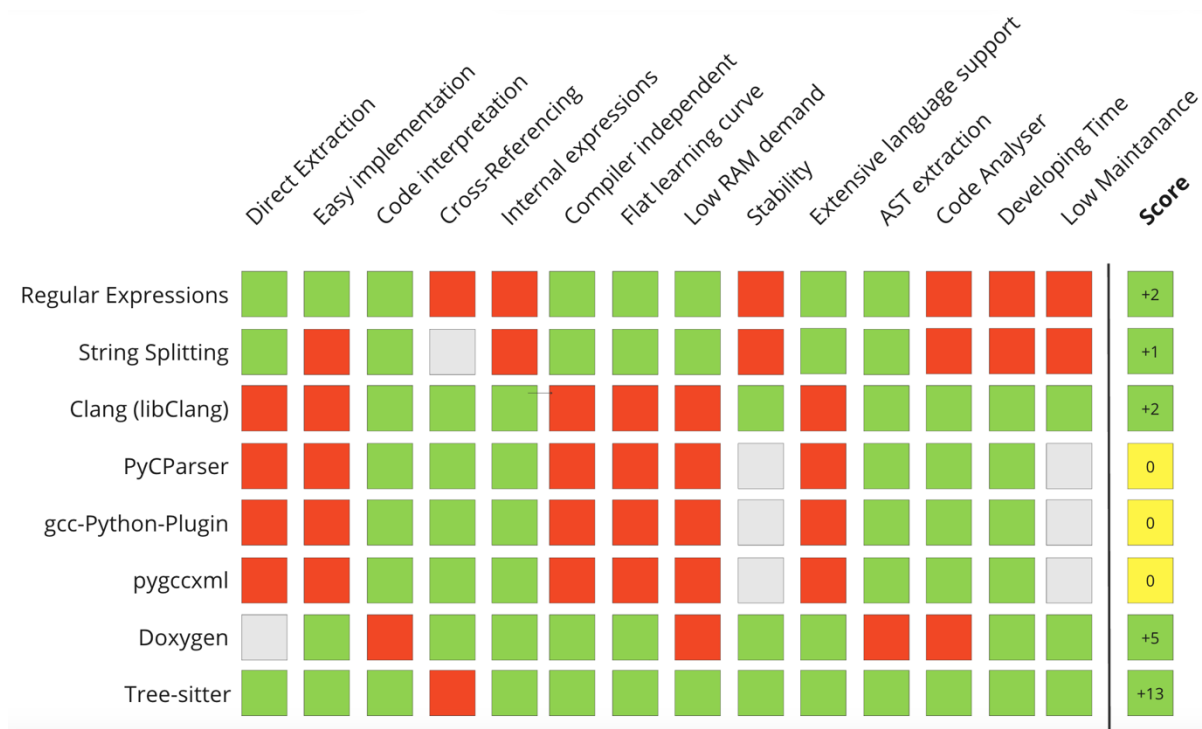
Figure 5: Overview-matrix summarizing the comparison of the dependency graph methods, where red equals -1 and green +1, grey fields neither add nor subtract to the score
