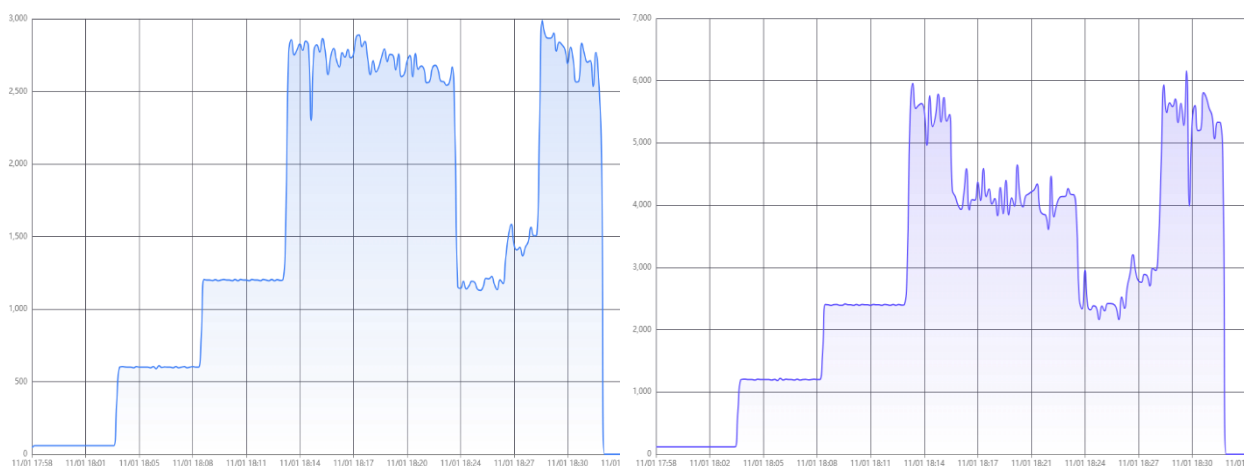
Figure 4: The message throughput of the broker during one of the latencies measurement tests. To the left is the total number of incoming messages per 30 seconds and to the right is the total number of outgoing messages per 30 seconds.
